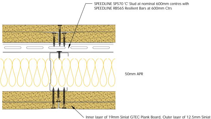
GTEC Standard Board, fixed with SPEEDLINE Drywall Screws at 300mm centres (200mm centres at external angles). Ref to table for fixing length.
